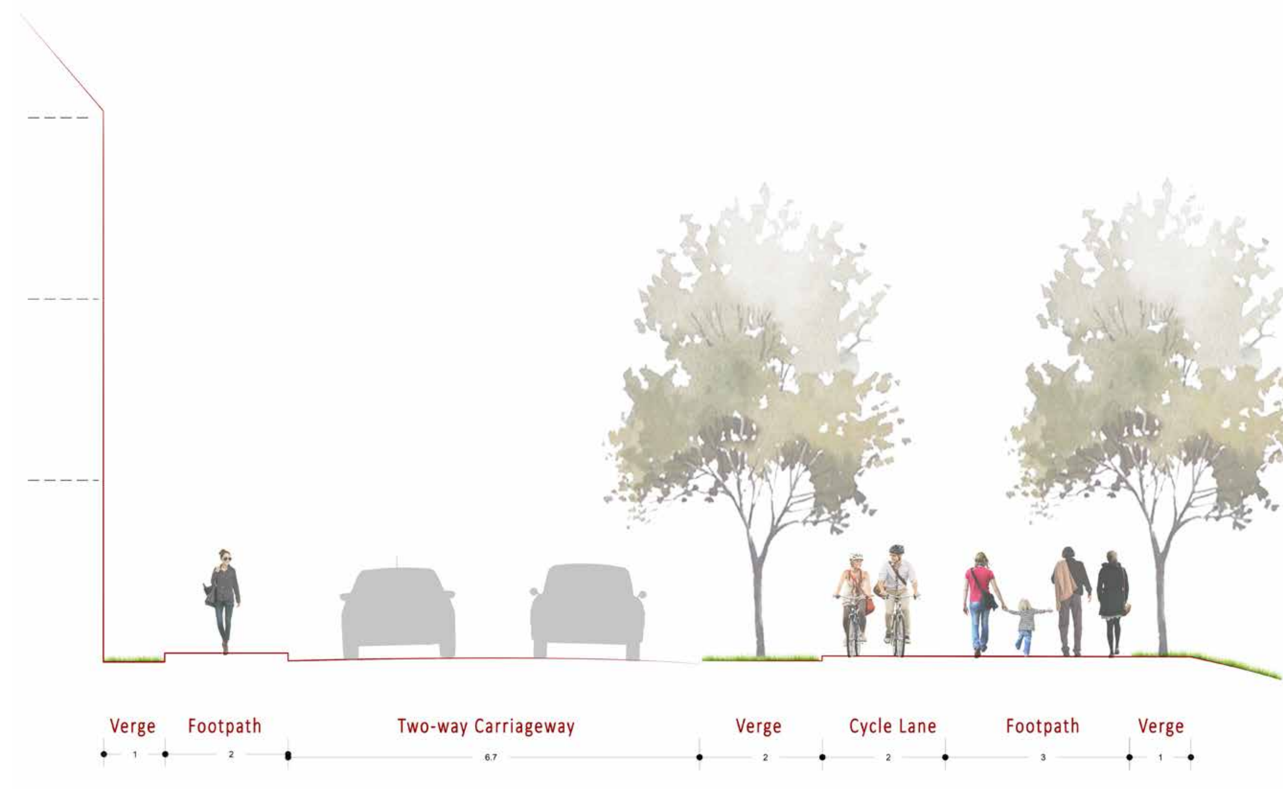
Typical Section of proposed Central Boulevard
